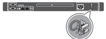
**4** Loop and secure the power cable using the retention strap.
